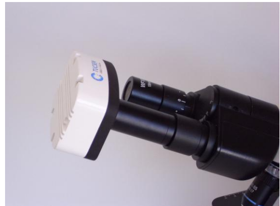
ISH camera mounted on binocular microscope with TCN eyepiece adapter
